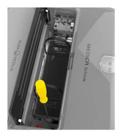
Step 4 - Switching on the unit and deactivate the system bypass Valves
